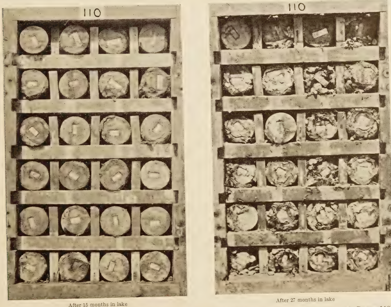
FIGURE 2.—CONDITION OF UNTREATED 1:1½:3 CONCRETE CYLINDERS OF MEDIUM CONSISTENCY (BATCH 1, CRATE 110) AFTER 15 AND 27 MONTHS IN MEDICINE LAKE, S. DAK. CURING SAME AS IN FIGURE 1
